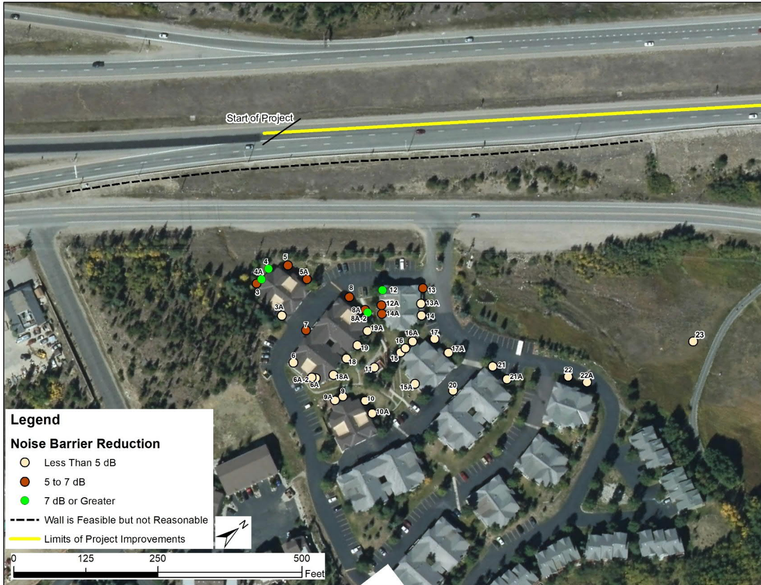
Figure 6A Interstate 70 EB Auxiliary Lane Noise Barrier EB-1 Location
