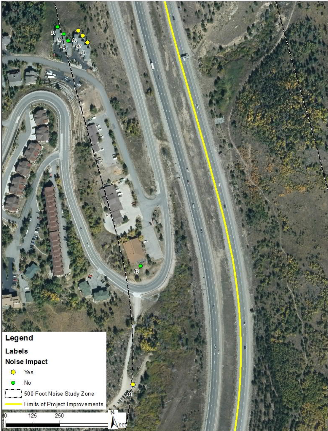
Figure 5B Roadways and Receiver Noise Levels for Design Year (2045) Proposed Action (Impacts Identified)
