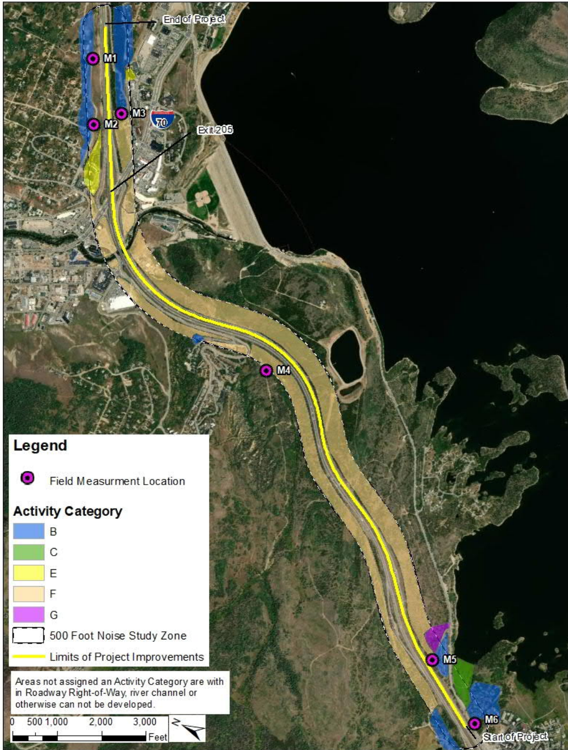
Figure 2 Interstate 70 EB Auxiliary Noise Study Zone, Activity Categories, and Noise Measurement Locations
