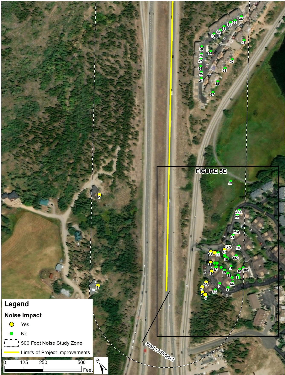
Figure 5A Roadways and Receiver Noise Levels for Design Year (2045) Proposed Action (Impacts Identified)
