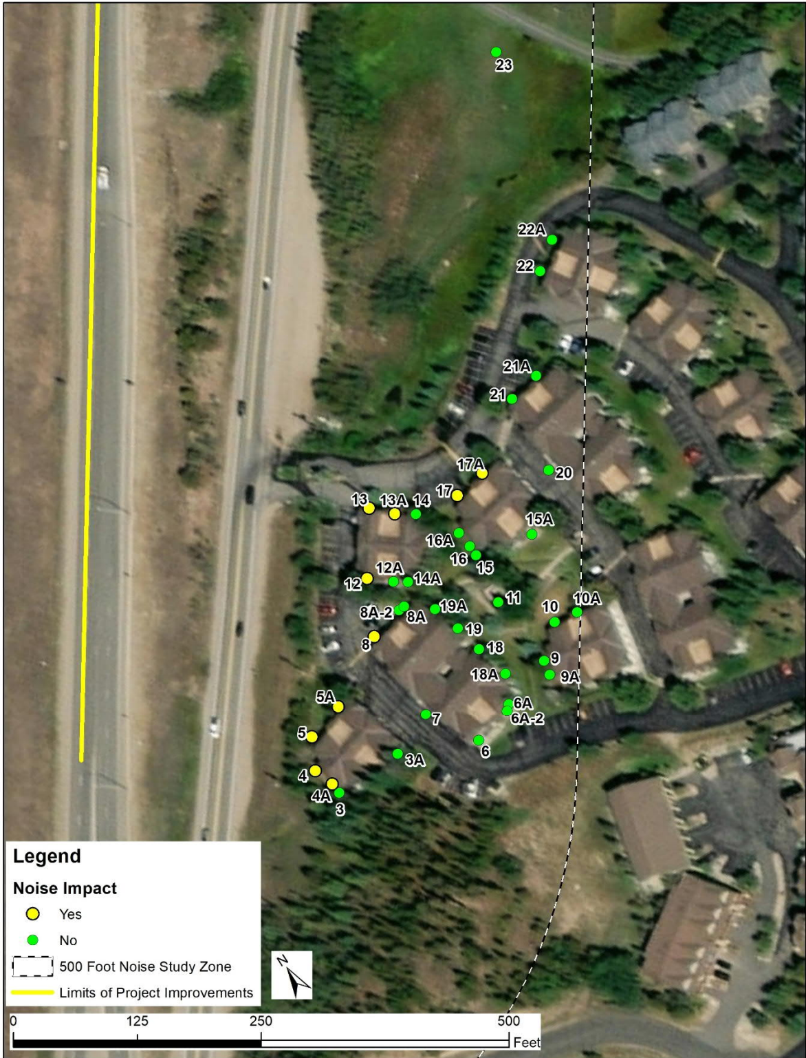
Figure 5E Roadways and Receiver Noise Levels for Design Year (2045) Proposed Action (Impacts Identified)
