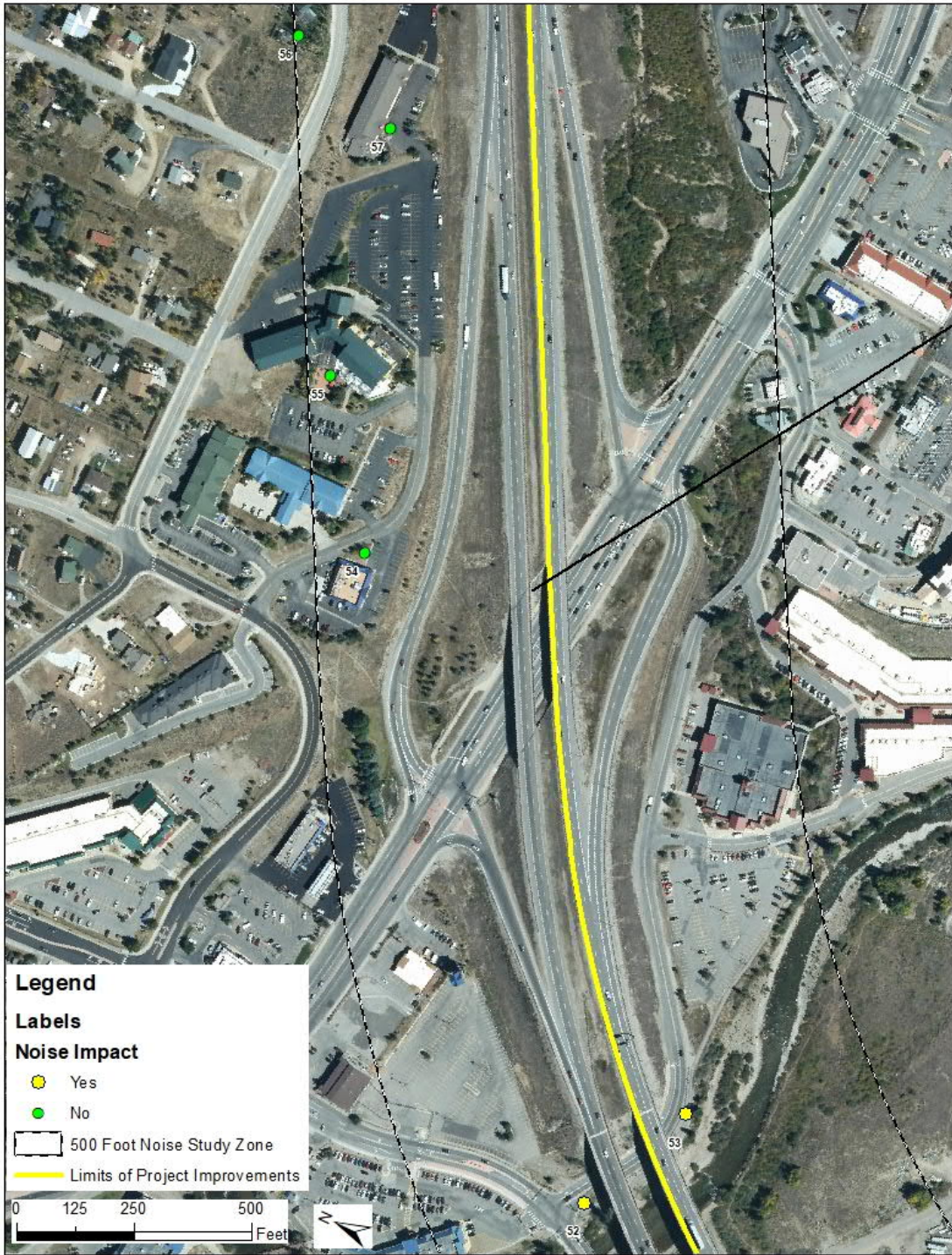
Figure 5C Roadways and Receiver Noise Levels for Design Year (2045) Proposed Action (Impacts Identified)
